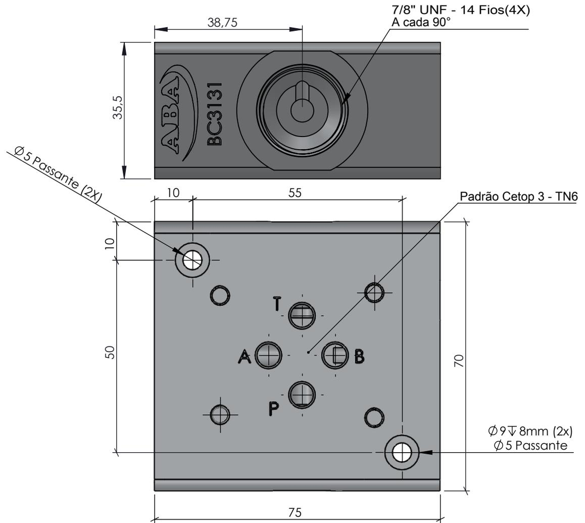
Torque Roscas 7/8" UNF: 50 Nm
