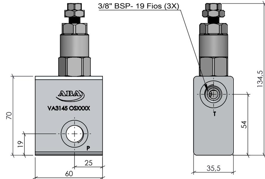
Torque Roscas 3/8" BSP: 35 Nm
