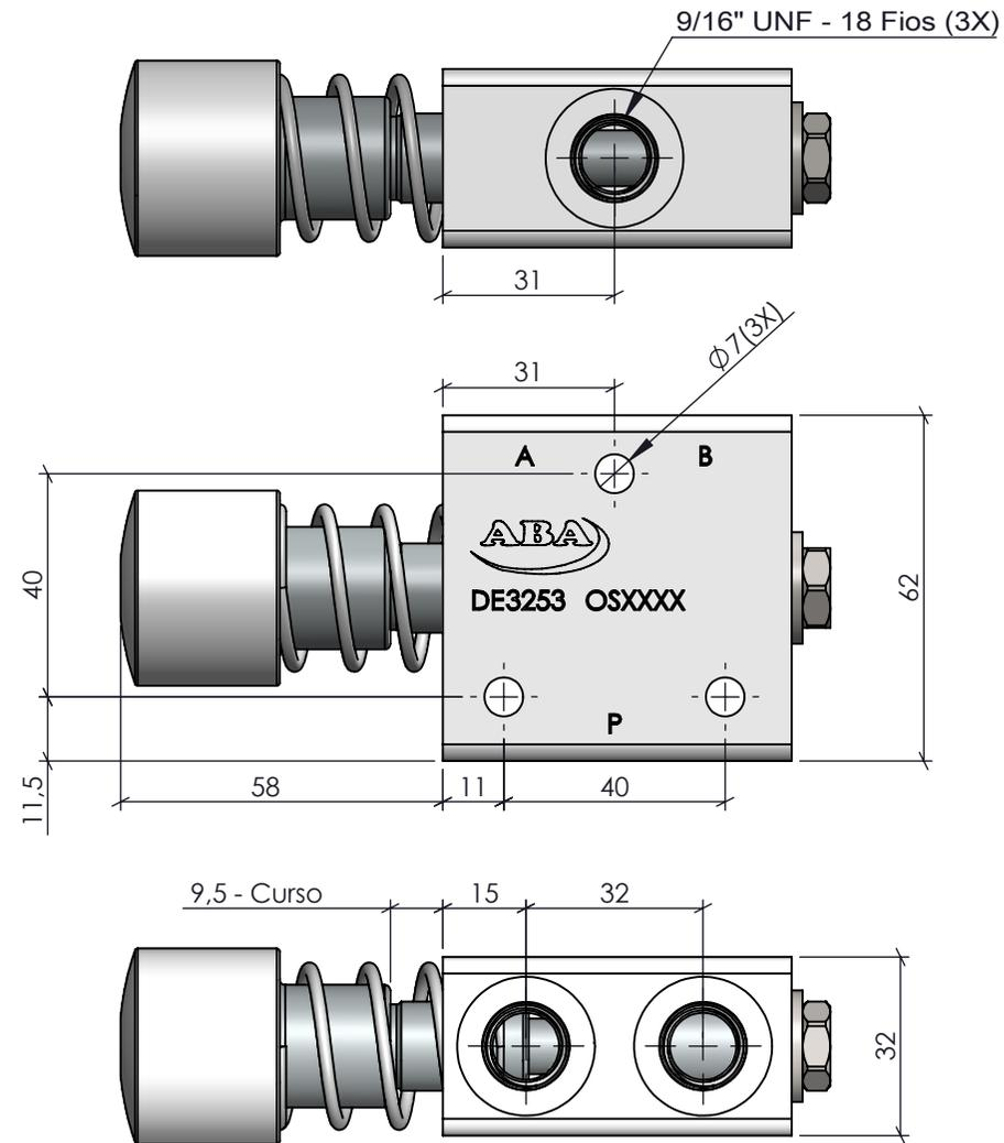
Torque Roscas 9/16" UNF: 30 Nm
