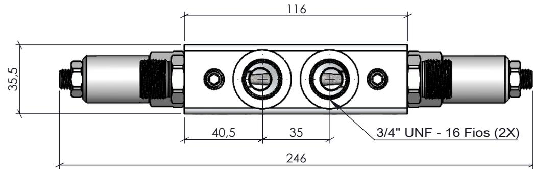
Torque Roscas 3/4" UNF: 35 Nm
