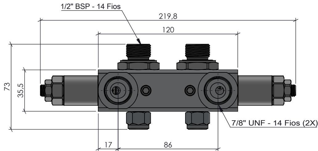
Torque Roscas 7/8" UNF: 50 Nm
