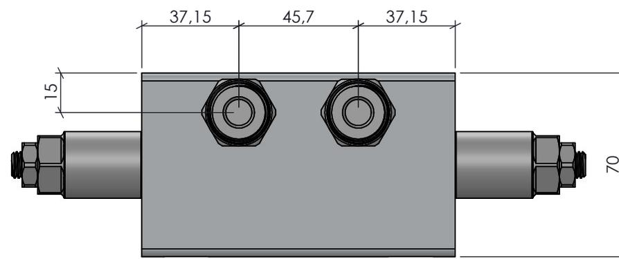
Torque Roscas 7/8" UNF: 50 Nm
