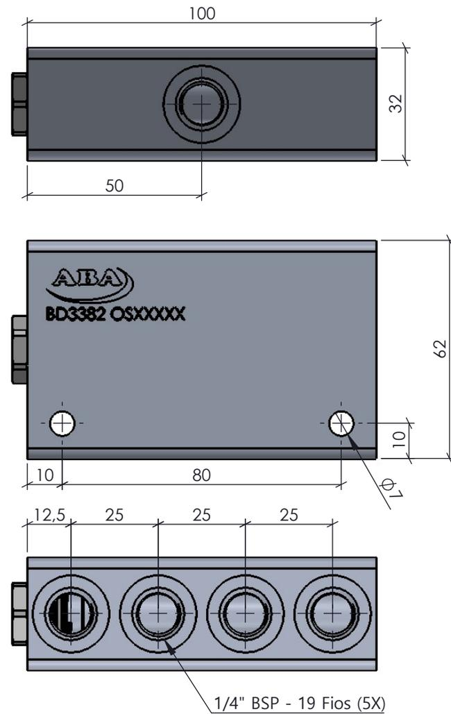
**Torque Roscas 1/4" BSP: 30 Nm**
